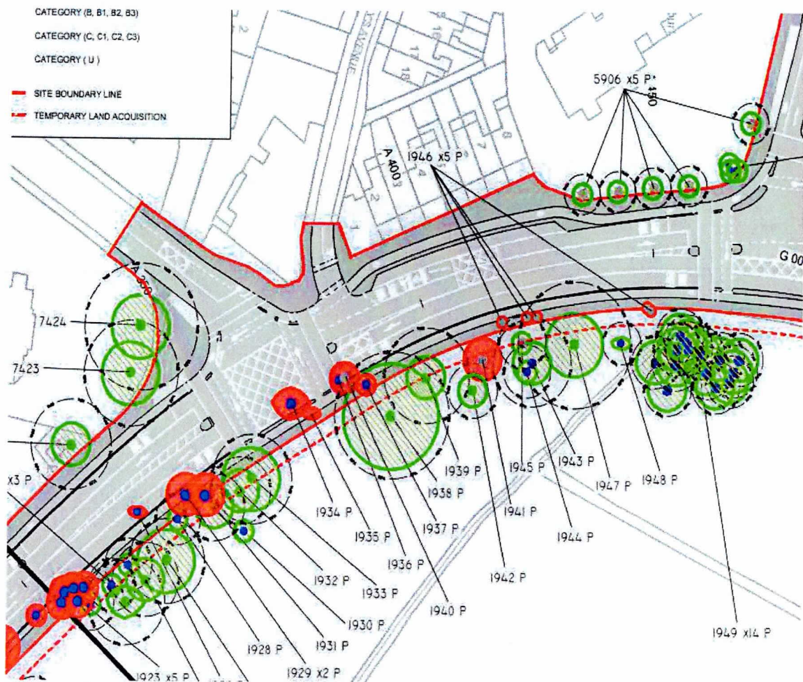
Figure shows the arboricultural tree protection plan of the same location as above and shows some of the calculated root zones of these trees to be retained extending out into the area where surfaces and services have to be installed.
