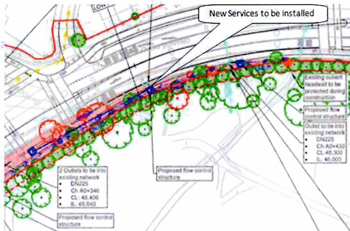
Figure 10 Image 1: shows services to be installed in the footpath & Cycle path outside the position of the new boundary wall, within the rootzone of trees scheduled for retention.
